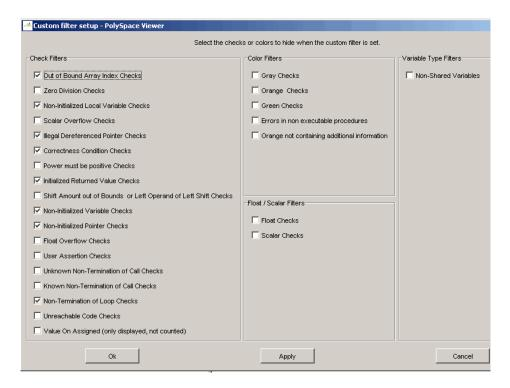
**3** Clear the filters for the checks that you want to display. For example, if you clear the **Out of Bound Array Index Checks** box, these checks display.
