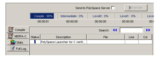
The progress bar highlights the current phase in blue and displays the amount of time and completion percentage for that phase.
