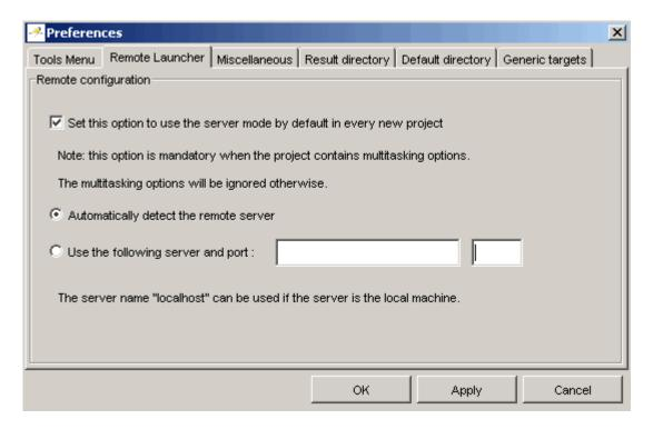
By default, PolySpace software automatically finds the server. You can specify the server by selecting **Use the following server and port** and providing the server name and port. For information about setting up a server, see the *PolySpace Installation Guide*.
