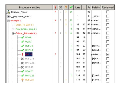
The check box for IDP.11 in Pointer Arithmetic() is selected because you selected the check box for this diagnostic in the current check view (upperright part of window).
