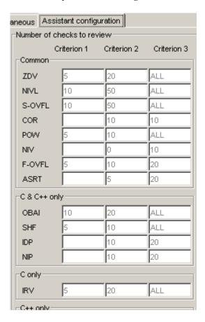
For example, the table specifies that you review five orange ZDV checks when you select criterion 1. The number of checks increases as you move from criterion 1 to criterion 3, reflecting the changing review requirements as you move through the development process.
