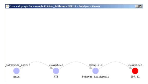
The code associated with IDP.11 is in Pointer\_Arithmetic. The generated main function calls RTE, which calls Pointer\_Arithmetic.
